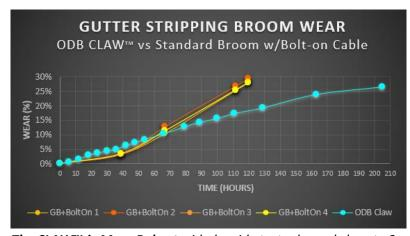
**The CLAW™** is More Robust; side-by-side tests showed close to 2 times longer expected functional service life, and on-the-street comparison have validated the testing data.
