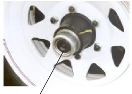
Grease fitting is behind rubber plug
