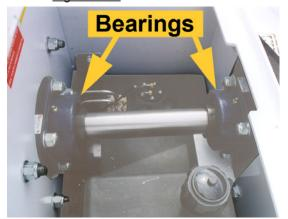
**NOTE:** DO NOT mix different types of grease. The old grease MUST BE purged before a different type of grease is used. Mixing grease WILL cause premature failure to the bearings.
