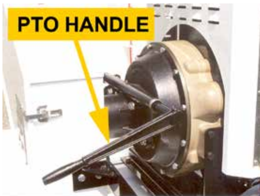
PTO shown disengaged
