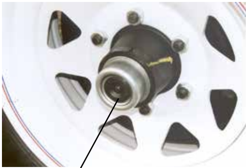
Grease fitting is behind rubber plug
