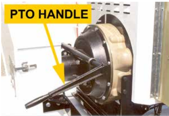
PTO shown disengaged
