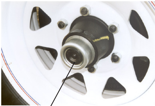
Grease fitting is behind rubber plug
