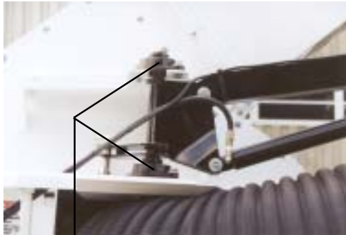
One fitting on each bearing
